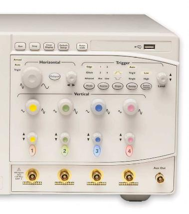
Hands-free operation with the Infiniium VoiceControl option. Just speak into the microphone to operate front-panel controls. **Segmented memory acquisition mode captures** bursting signals at maximum sample rate without consuming memory during periods of inactivity.
